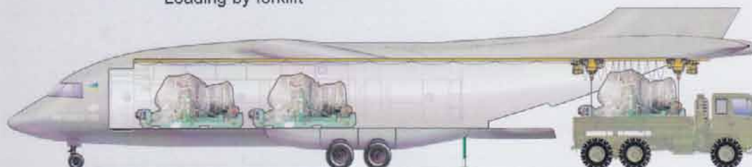
Loading the turbojet engine by upper handling equipment (option), max. cargo weight up to 8 t
