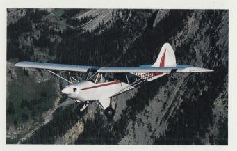
The HUSKY can be routinely flown for as long as seven hours at speeds in excess of 110 mph. Required take-off run is less than 250 ft and landing distance with full flaps is less than 350 ft. Initial rate of climb is greater than 1500 ft/min and the service ceiling is in excess of 20,000 ft.
