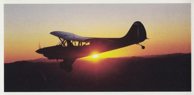
The HUSKY features a Clark Y/USA 35B airfoil which is modified extensively to provide high-lift and docile stall characteristics, and which is combined with long-span single-slot manually-operated flaps to provide outstanding slow-flight capabilities and exceptionally short take-off and landing distances.
