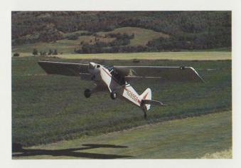
Proven utility aircraft design concepts have been integrated with time-tested construction materials and techniques in the HUSKY to produce a high-performance aircraft with extraordinary utility features. The high-lift wing, large area flaps, 180 hp engine, and constant-speed propeller combine to provide exceptional short field performance and impressive slow-flight characteristics.
