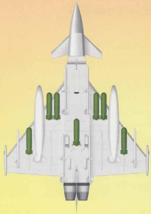
Typical Air-to-Surface configuration
