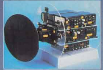
The ECR 90 Advanced Multi-Mode Pulse Doppler Radar
