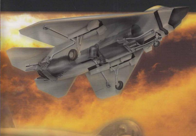
The complex STOVL requirement demands an uncomplicated solution – a simple, deployable direct-lift propulsion system. Lift nozzles are hidden within the airframe. They are coupled with a three-axis attitude control system – similar to the AV-8B – to give the Boeing JSF its short takeoff and vertical landing capability. It is a proven, light-weight, low-risk concept that provides seamless transitions between jet-borne and wing-borne flight within 2 seconds and at full power.
