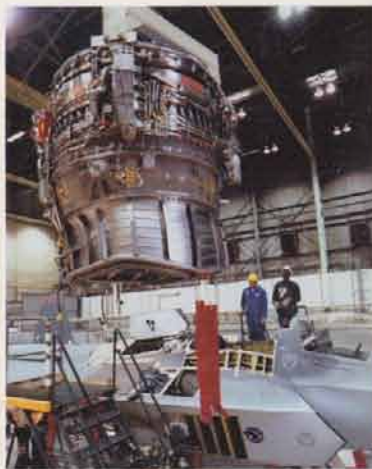
Late last year, the short-driven lift fan was installed in the X-35B short takeoff, vertical landing demonstrator at Lockheed Martin's Palmdale, Calif., facility. The lift fan installation includes the fan, a vectored nozzle, clutch, and all actuation and service systems in an integrated unit.
