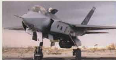
The X-35B is shown here during hover pit testing (and before the tails were repainted) earlier this spring. The open lift fan doors, open auxiliary inlet doors, and the downturned engine exhaust nozzle can be seen clearly.
