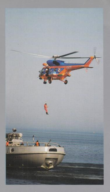
Lifting the shipwrecked persons can be carried out using rescue belts, rescue basket for 2 persons or stretchers. The stretchers used on ANACONDA (PARAMEDICS RESCUE PACK) can be lifted in both horizontal or vertical position, and they can be folded for transport.
