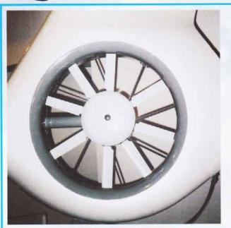
New generation "Fenestron" with new airfoil and asymmetrical blade spacing (8 blades) for low noise emission.
