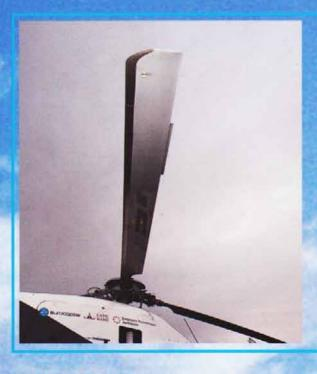
The composite main rotor blades are of fail safe design:
