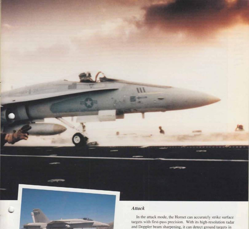
In the attack mode, the Hornet can accurately strike surface targets with first-pass precision. With its high-resolution radar and Doppler beam sharpening, it can detect ground targets in adverse weather and at night. Both free-fall and guided weapons can be delivered with pinpoint accuracy. The nine payload stations on the wings and fuselage allow the Hornet to carry various combinations of bombs, missiles and external fuel tanks.
