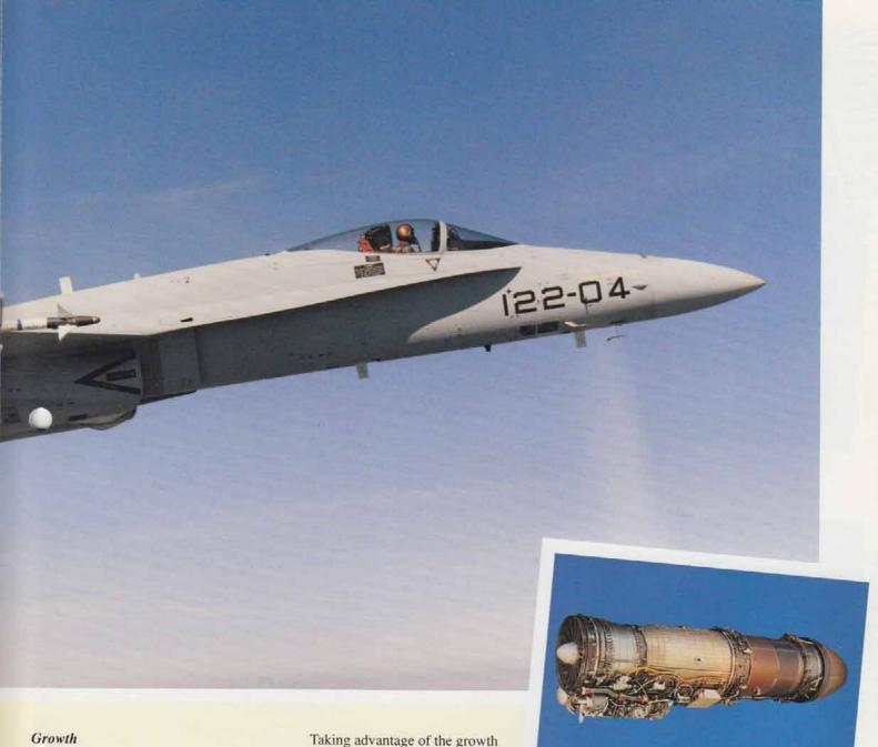
Hornet designers integrated critical growth potential into the F/A-18. With minimum modifications, about 12 cubic feet are available for future avionics and new systems.
