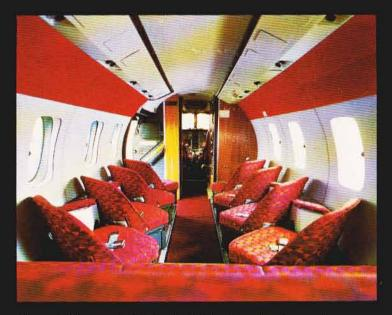
The eight comfortable individual seats have been arranged at an angle to afford each passenger a maximum of leg-room. Each seat is 19,5 inches wide, or the size of a normal first-class seat. Four additional passengers have space on the couch at the rear of the cabin.
