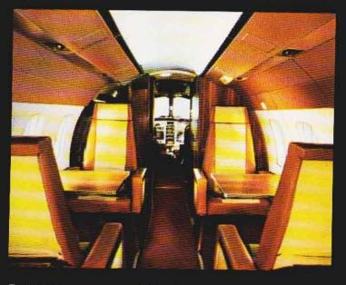
Each seating accommodation is equipped with a complete service panel, with fresh-air nozzle, reading lamp and oxygen mask. Connections for telephones and tape recorders can easily be installed.
